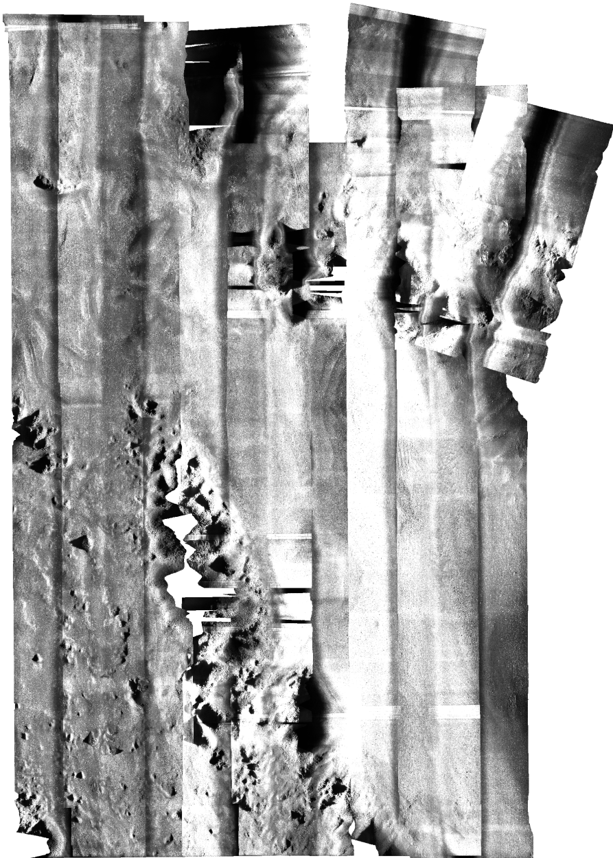
Figure 5.3: Sonar mosaic of the Nord-Leksa coral reef. The resolution is 33x33 cm, covering an area of 1325x2180 m \approx 2.9 \text{ km}^2 . The image was created in Reflection, with the "average" mapping option. This option merges overlapping areas such that the nadir disappears and the complete area can be inspected. Some holes appear where shadows have prevented the sonar from collecting data. The image does not cover the entire dataset.
