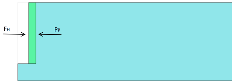
Figure 5.20: Horizontal forces acting on the wall
