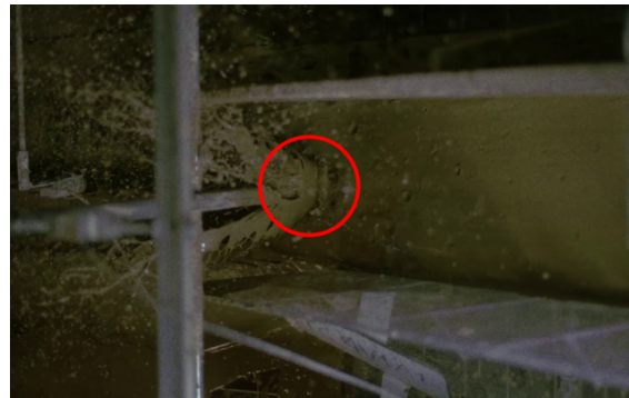
(c) Impact of the soil clump on the force sensor.
