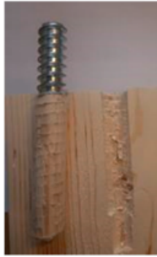
Figure 3.33: Interface plane between wood and rod [14]
