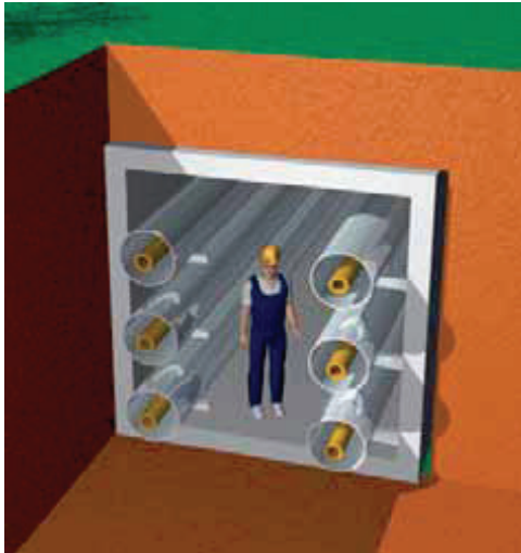
Figure 9: Illustration of GIL tunnel. (Source: Siemens)
