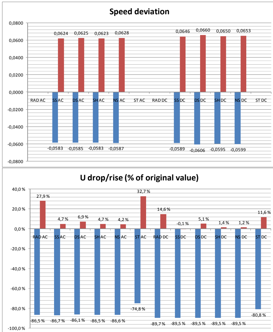
Figure 72 –Fault scenario two. Maximum speed deviation [pu on system base] and voltage deviation [% of initial value] of the wind turbine generator closest to the substation when the fault occurs in the same feeder as the generator is placed.
