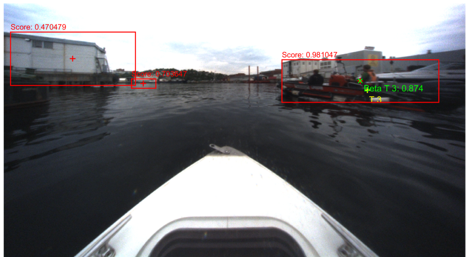
Figure 5.22: Computed association probabilities for image detection, scenario 5.
