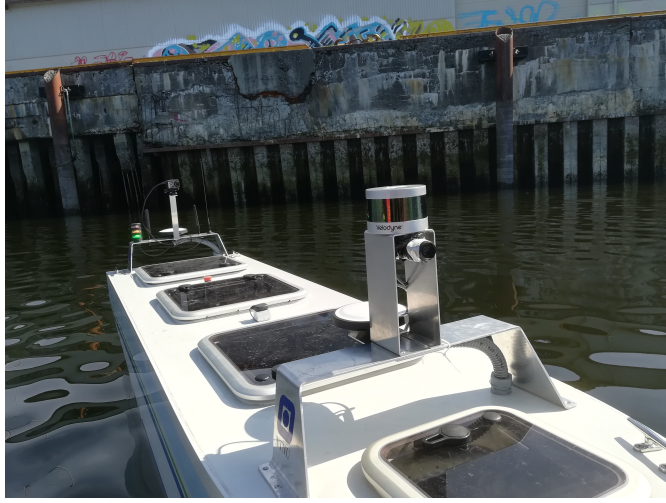
Figure 4.4: The camera and lidar mounted together on the ReVolt scale model ship.
