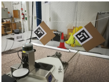
Figure 4.7: The lidar-camera calibration setup.
