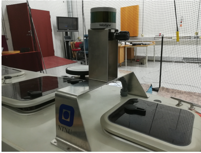
Figure 4.1: The sensor mounting bracket on the fore targa hoop.
