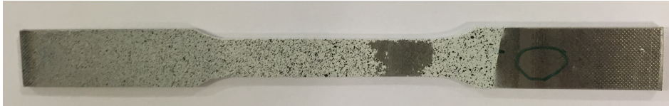
Figure 3.2: Plane test specimen similar to the one used for the tensile test
