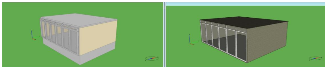
FIGURE 183: IDA ICE – CURTAIN WALL – TYPE: STOREFRONT – LEFT: IFC MODEL. RIGHT: ENERGY MODEL
