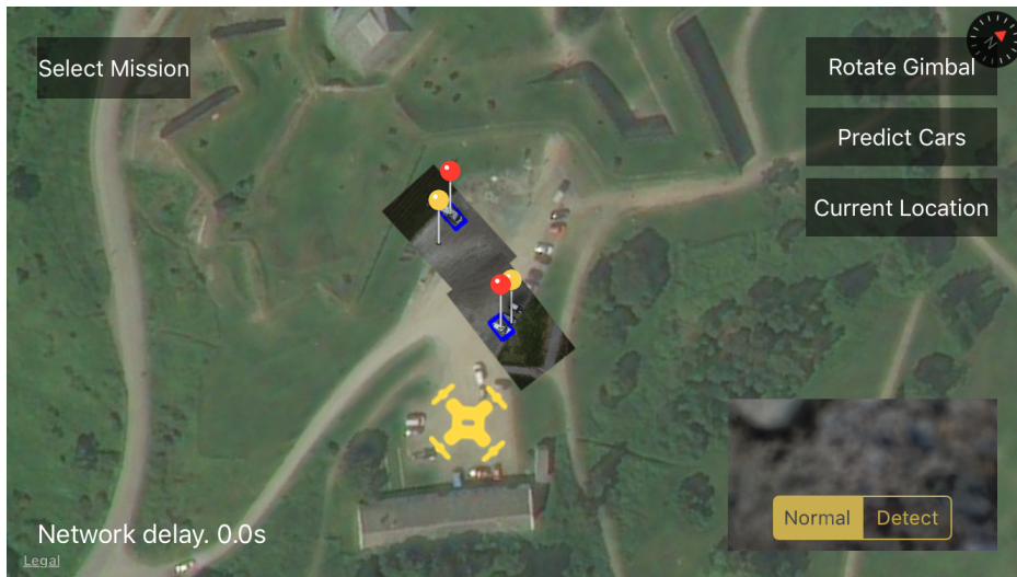
Figure 4.18: The predicted locations of the cars on top of the projected overlay. The predicted locations are given with red pins.
