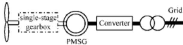
Figure 7: Scheme of a single-stage drive PMSG system with a full-scale converter [12]
