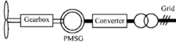
Figure 8: Scheme of a single-stage drive PMSG system with a full-scale converter [12]
