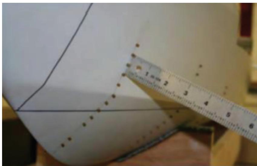
Figure 3.1: Studs on a ship model (Murphy (2010)).
