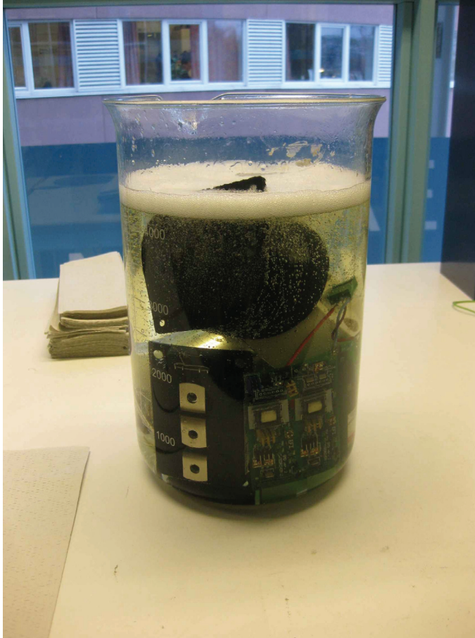
Figure 53 Picture of the oil-filled glass with tested components inside [32]
