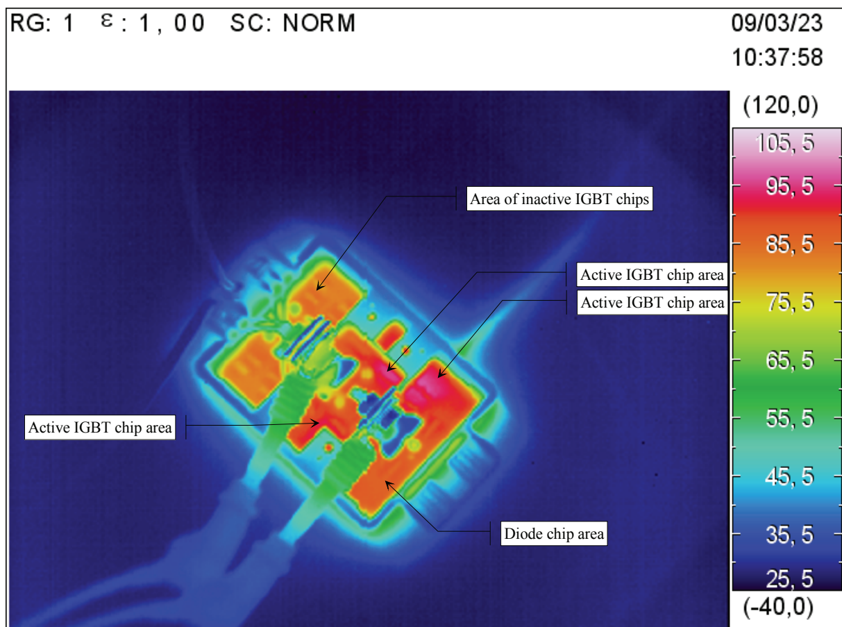
Figure 41 Thermocamera image of the IGBT module in thermal steady state
