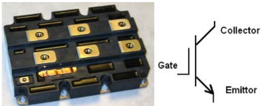
Figure 2-21: Power IGBT (3300V, 1200A) and symbol
