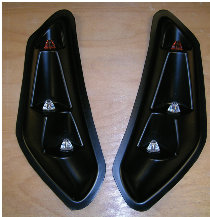
Figure 39: Holders with the lenses for the front lights.
