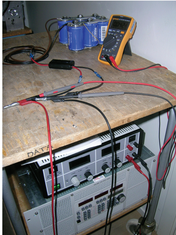
Figure 59: Shows the setup used when testing the supercapacitor module. A “Watt’s up” energy measurement device is used to register necessary Wh and Ah ratings.
