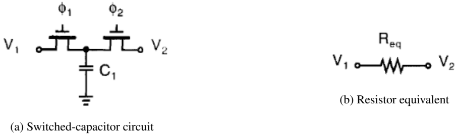
Figure 2.7: Resistor equivalence of switched capacitor capacitor
