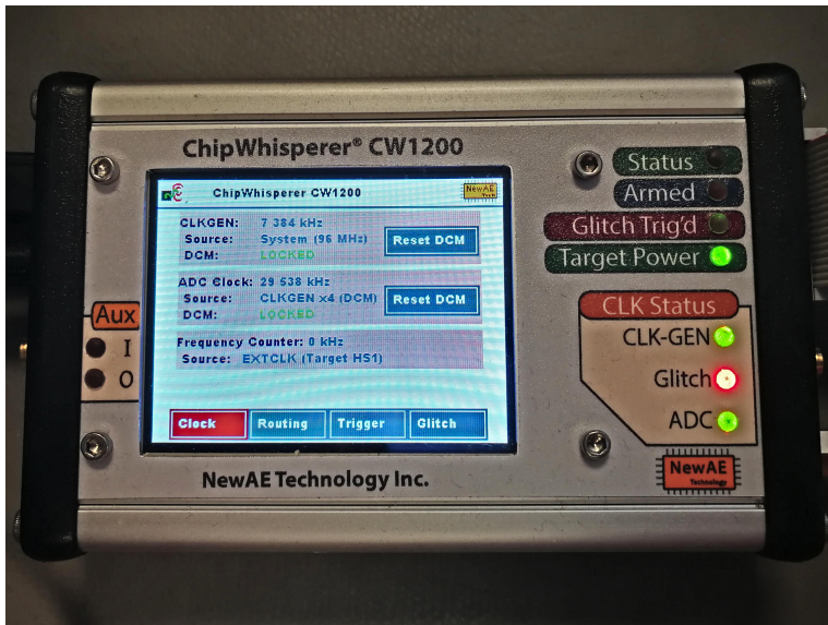
Figure 5.2: CW1200 ChipWhisperer Pro. Used to measure power and communicate with different MCUs under attack.
