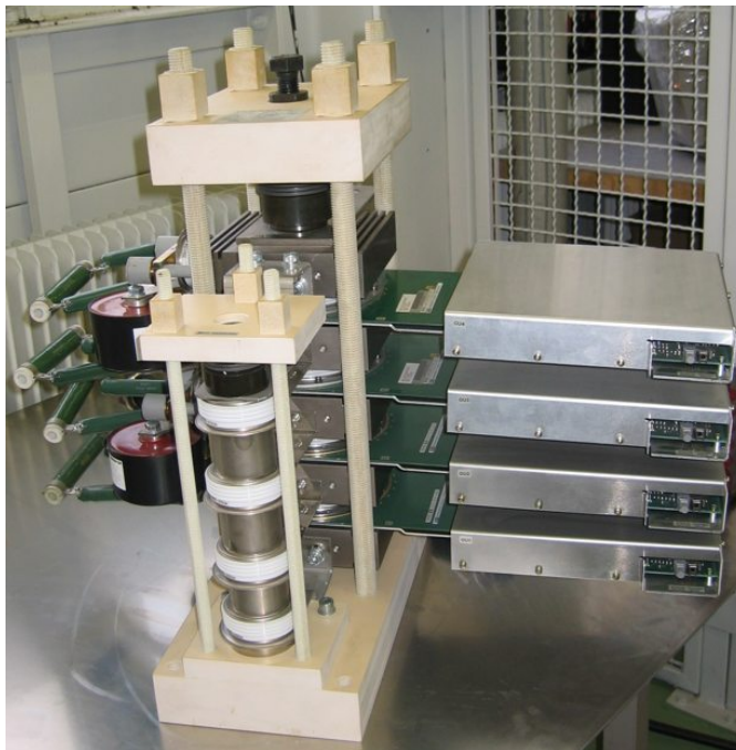
Figure 6.9: 4xIGCT ABB switch
