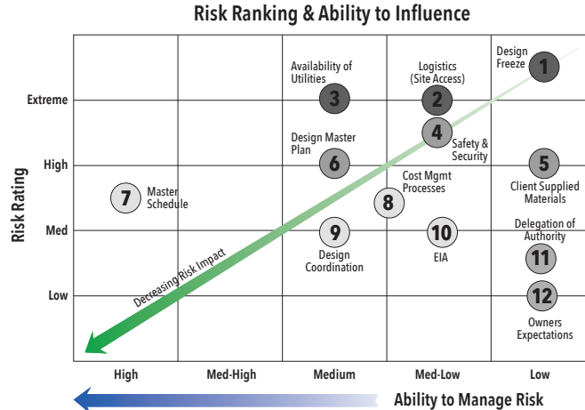
Figure 1. Risk ranking and ability to influence: Derek A. Price, Parsons Brinckerhoff presented at INCOSE 2004
