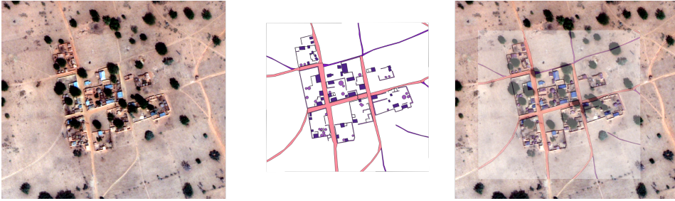
Figure 3.1: Ground truth labels and aerial image from the Dstl Satellite Imagery Feature Detection
