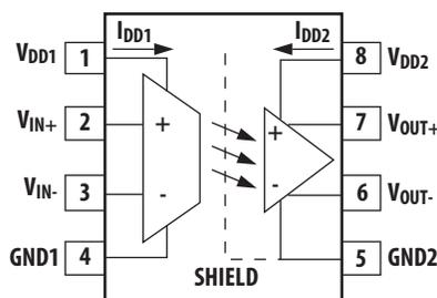
The connection of a 0.1 μF bypass capacitor between pins 1 and 4, pins 5 and 8 is recommended.
