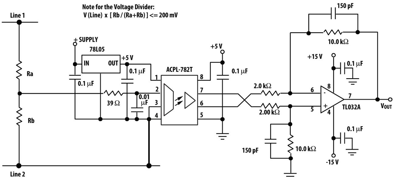
Figure 21. Recommended circuit for voltage sensing application.
