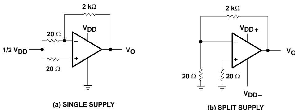
Figure 2. Noise-Test Circuit
