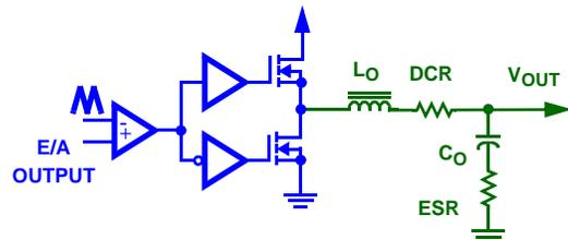
$$GAIN_{OPENLOOP} = \frac{V_{IN}}{\Delta V_{OSC}} \cdot \frac{1 + s \cdot ESR \cdot C_{OUT}}{1 + s \cdot (ESR + DCR) \cdot C_{OUT} + s^2 \cdot L_{OUT} \cdot C_{OUT}}$$
