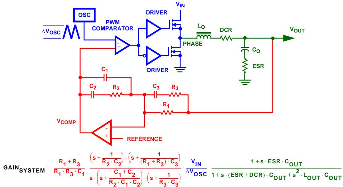
FIGURE 10. CLOSED LOOP SYSTEM WITH TYPE III NETWORK
