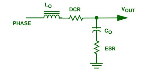
$$GAIN_{FILTER} = \frac{1 + s \cdot ESR \cdot C_{OUT}}{1 + s \cdot (ESR + DCR) \cdot C_{OUT} + s^2 \cdot L_{OUT} \cdot C_{OUT}}$$
