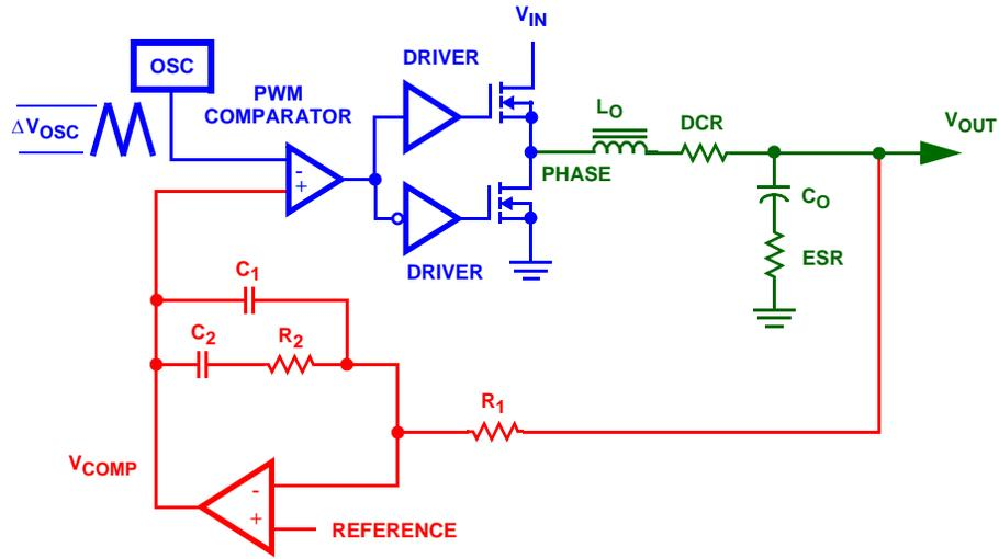
$$GAIN_{SYSTEM} = \frac{1}{R_1 \cdot C_1} \cdot \frac{\left(s + \frac{1}{R_2 \cdot C_2}\right)}{s \cdot \left(s + \frac{C_1 + C_2}{R_2 \cdot C_1 \cdot C_2}\right)} \cdot \frac{V_{IN}}{\Delta V_{OSC}} \cdot \frac{1 + s \cdot ESR \cdot C_{OUT}}{1 + s \cdot (ESR + DCR) \cdot C_{OUT} + s^2 \cdot L_{OUT} \cdot C_{OUT}}$$
