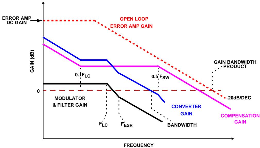
$$GAIN_{dB}(f) = GAIN_{MODULATOR} + GAIN_{FILTER} + GAIN_{TYPEII}$$
