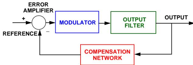
FIGURE 1. BASIC BLOCKS OF THE BUCK REGULATOR
