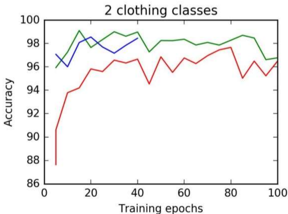
Figure 3.10: The red line shows the CNN’s test certainty multiplied by its averaged test success rate against the number of epochs with 0 image augmentation functions in use. The green line shows the resulting performance including the 4 transformation augmentations, and the blue line has all of the 8 augmentations including the lighting variations enabled.
