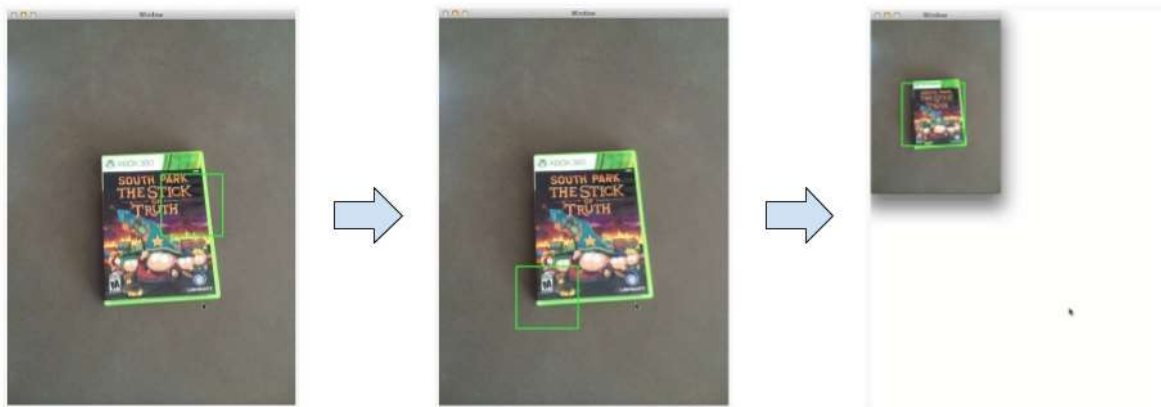
Figure 3.4: The sliding window algorithm and the image pyramid performed on an image of a video game cover, courtesy of Adrian Rosebrock [39]
