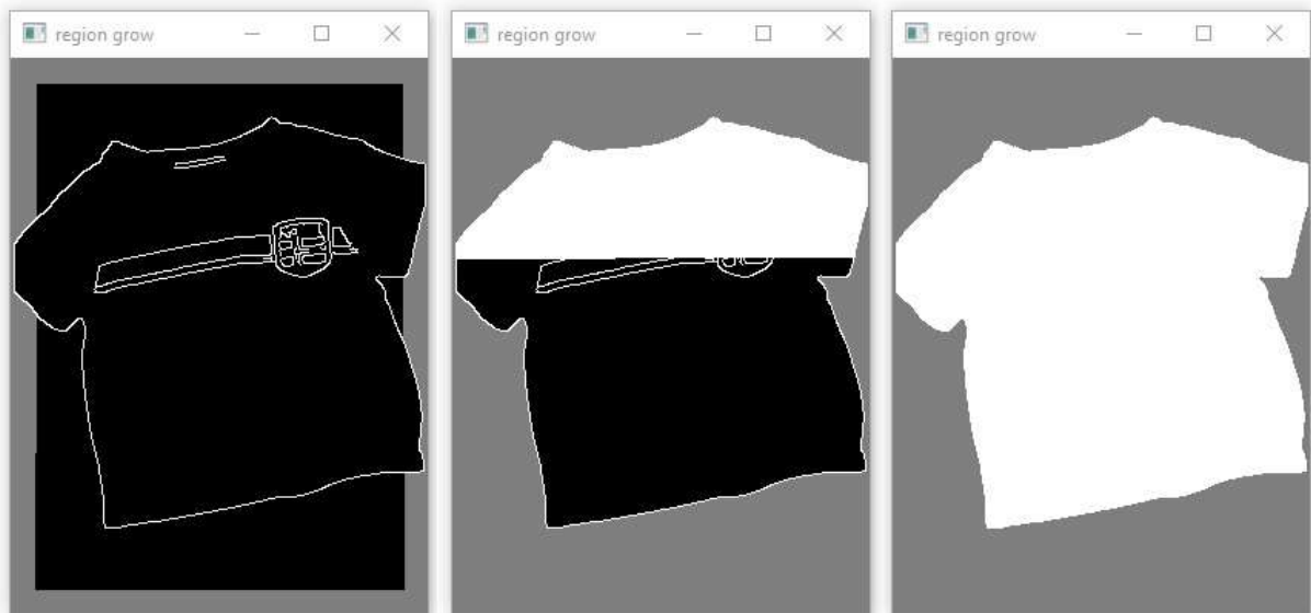
Figure 3.36: The region grow algorithm during runtime. The gray color illustrates the determined background pixels, black pixels are yet to be determined, and white represents the resulting foreground pixels.
