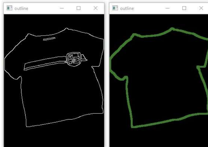
Figure 3.38: Outline extraction. The dilated outline of a Canny edge map is shown to the right in green.
