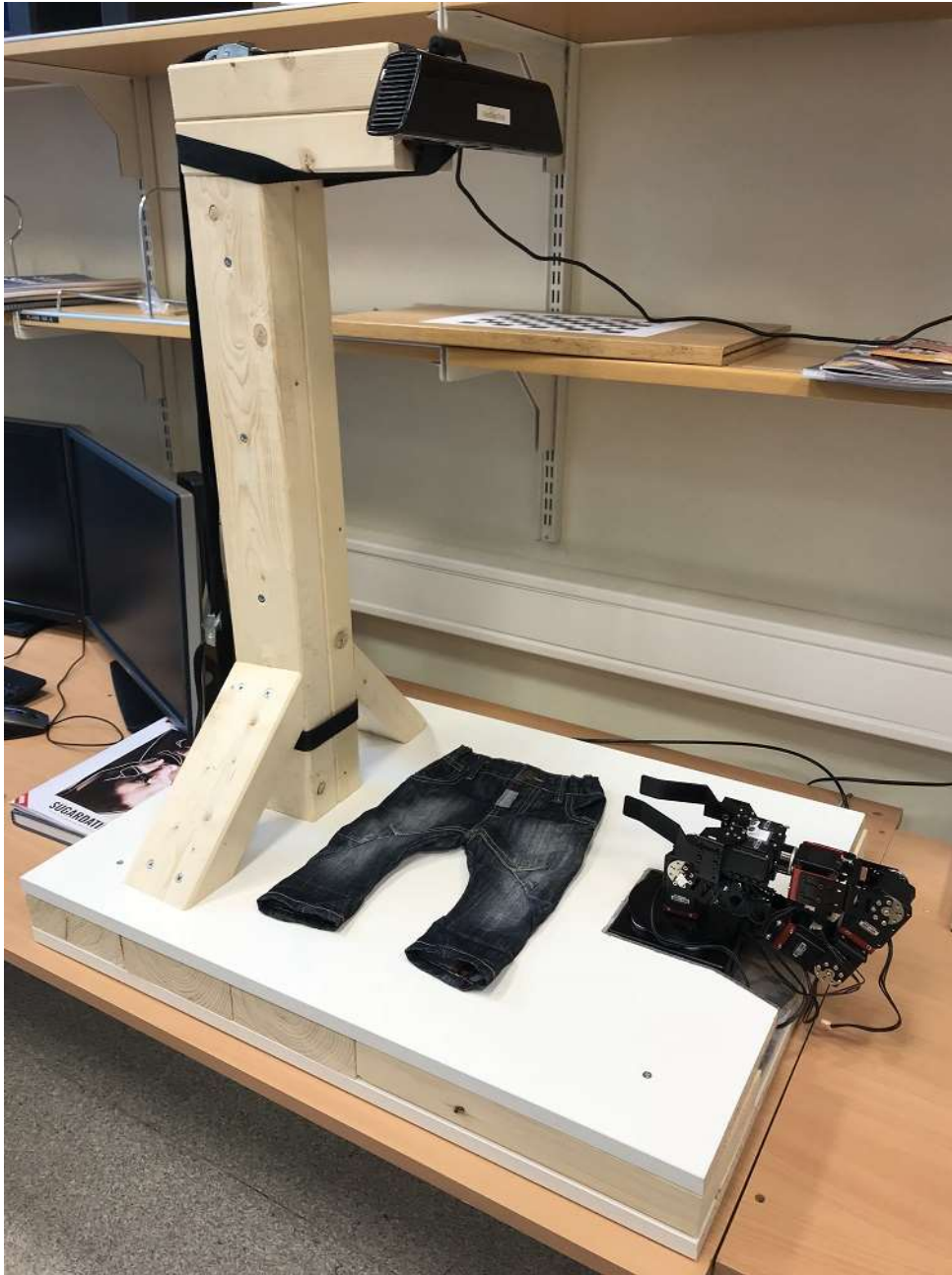
Figure 3.26: The Kinect camera was rigorously fastened to the camera mount support structure with baggage straps.
