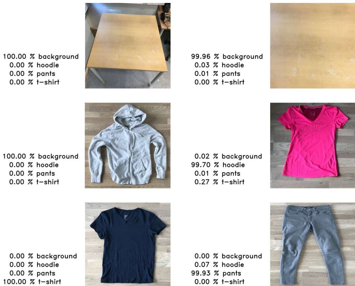
Figure 3.13: Examples of testing results produced after the inclusion of the 'background' category in the training data set
