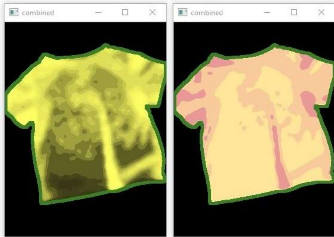
Figure 3.40: A depth image segmentation clustering similar pixel intensity values together by use of thresholding.
