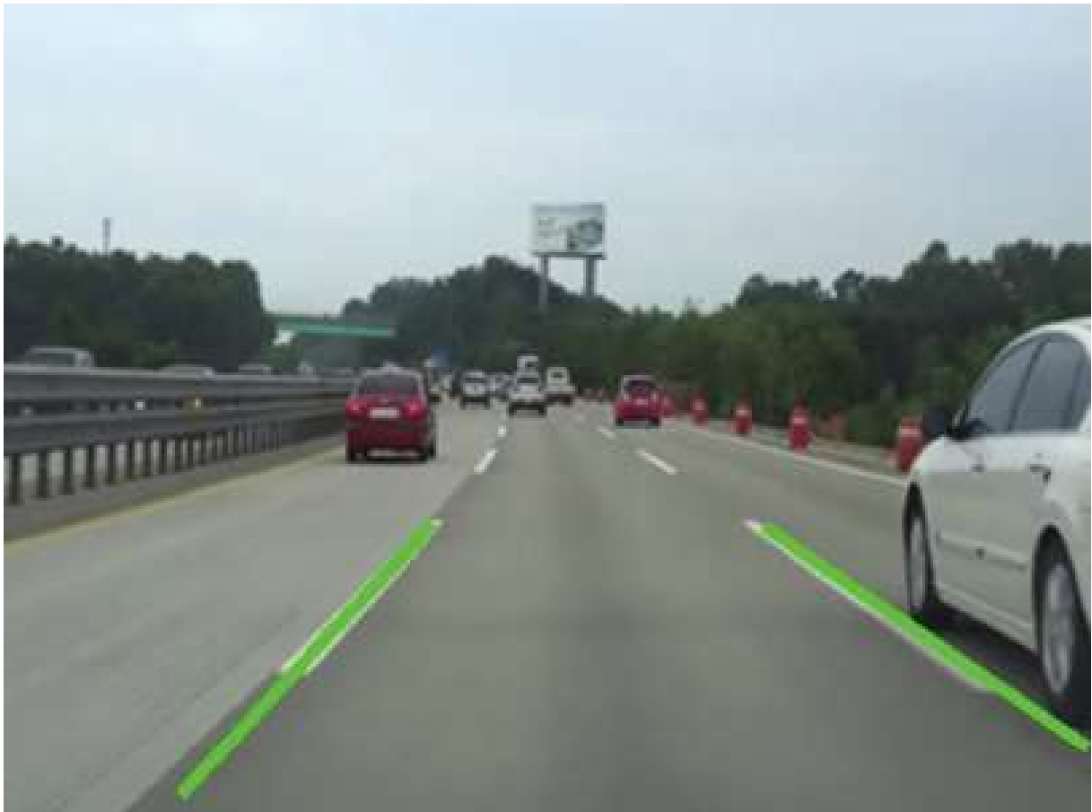
Figure 2.5: Example use of the local Hough transform for lane detection [30], a popular feature extraction method for detecting lines or circular features in images not discussed in this work.
