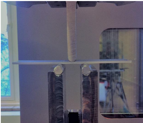
Fig.46 Before the bending test
