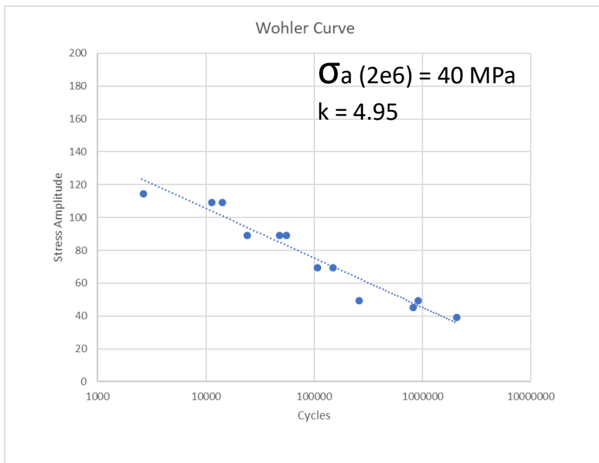
Fig.79 Fatigue curve of the welded specimens
