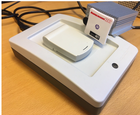
Figure 5.2: Setup of the experiment. The USRP is placed next to the RSE and the OBU, in order to receive a good signal power level.
