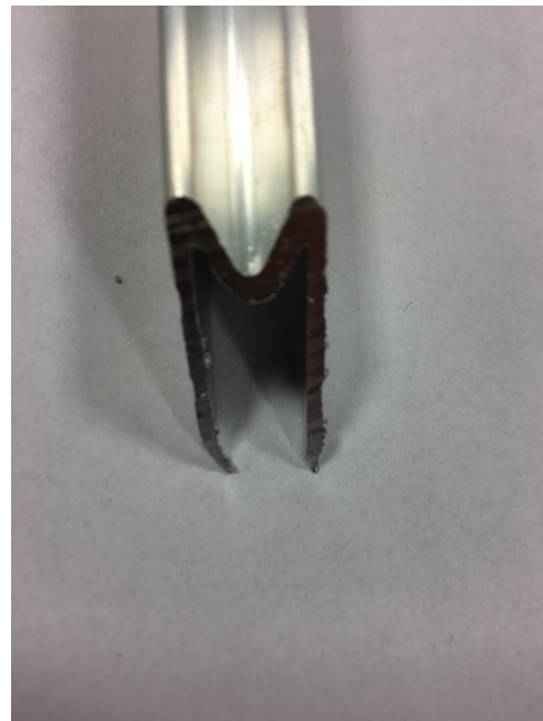
Figure 8.10: Profile bent after cut
