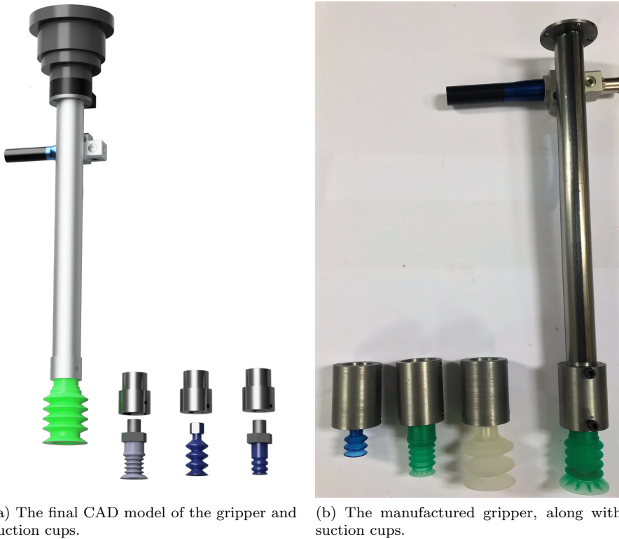
Figure 3.5: Illustration of the CAD design of the gripper and the manufactured product. The different suction cups are easy to change with the designed mounting system.
