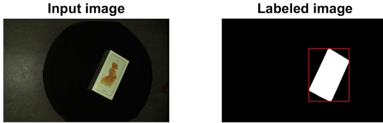
Figure 3.13: Illustration of the proposed bounding box region from the automated labeling program.
