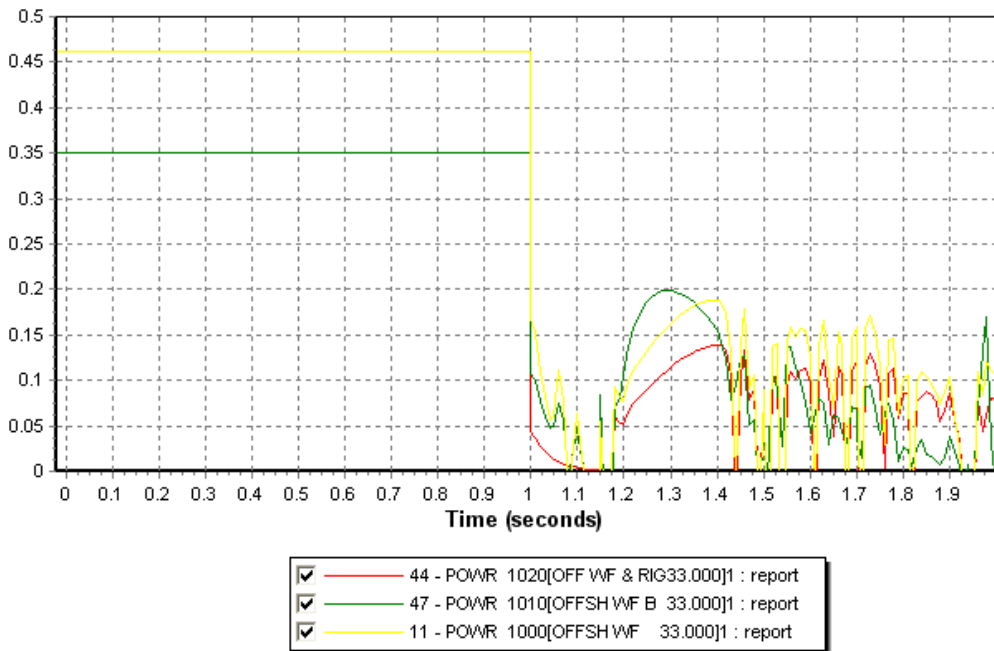
Figure 7-24: Power from the offshore generator, DFIG in red and yellow, FIG in green in pu on system base
