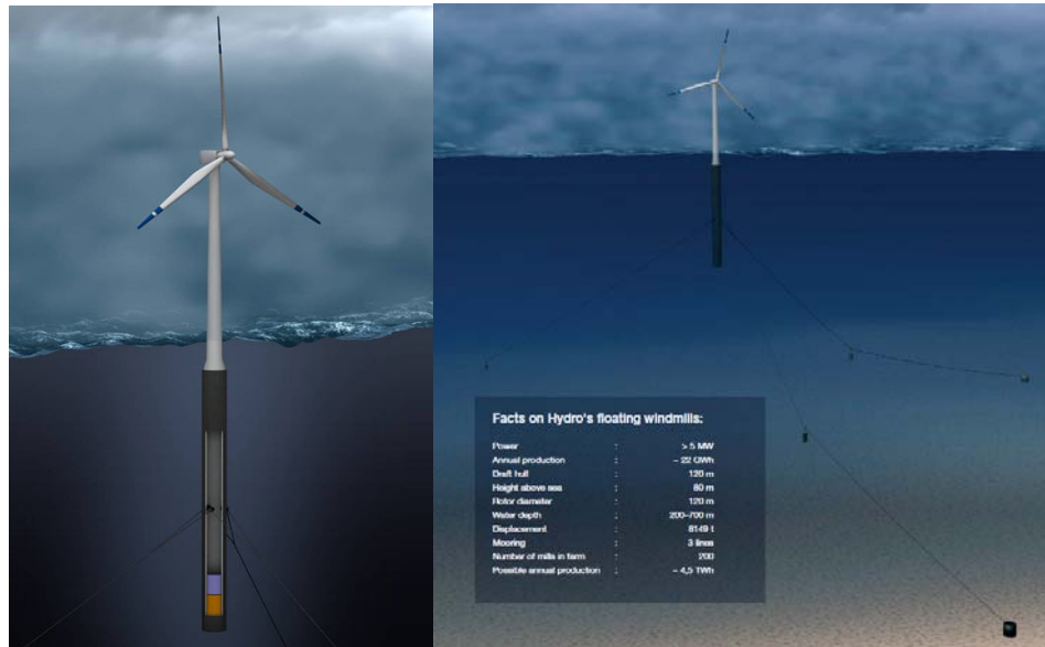
Figure 1-13: HYWIND project, detailed view on the ballast (left) and view on the mooring system (right)
