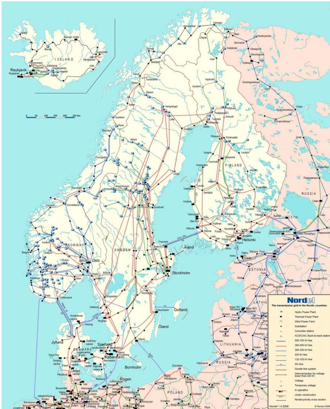
Figure 1-11: Nordic grid in the Nordel system: the HVDC transmissions crossing the seas are in blue
