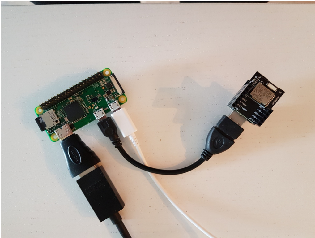
Figure 7.7: Hardware setup of the Raspberry Pi Zero W and the RFduino Host.
