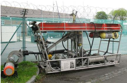
**(a)** Royal Navy's Cutlet ROV from the 1950s, which was used for recovery of torpedoes and mines
