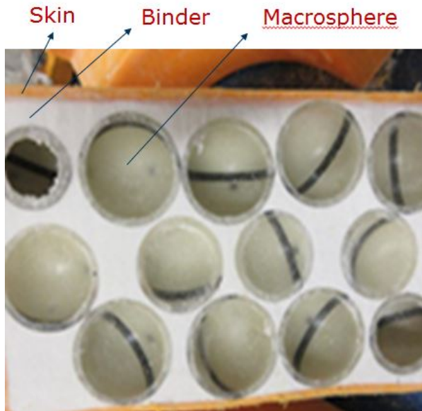
Figure 6.17: Cut-through Section of Composite Syntactic Foam
