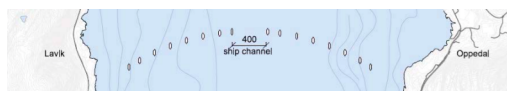
Figure 2.11: Bird's view of SFT for Sognefjorden showing pontoon and ship channel location (NPRA, 2012a)
