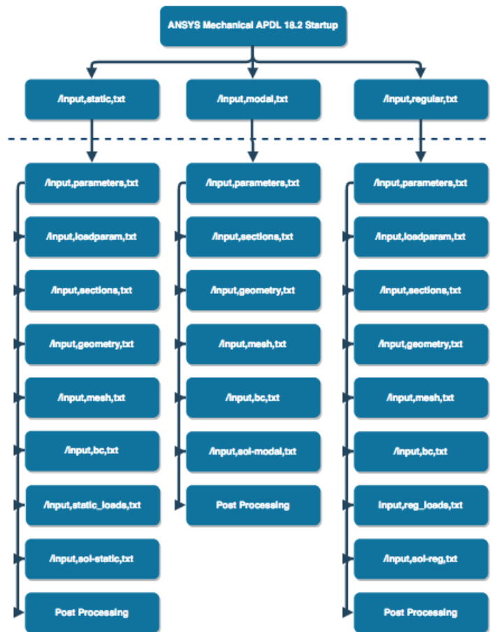
Figure 7.1: Flowchart of static, modal and regular wave analysis scripts setup in ANSYS Mechanical
