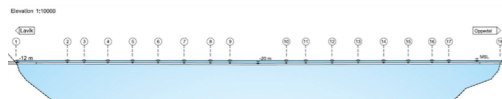
Figure 2.12: Side view of the SFT over the Sognefjord showing submerged pipe, pontoon and navigation channel (NPRA, 2012a)
