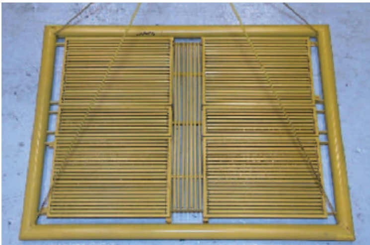
Figure 1.2: Example of porous structure, a protection cover for subsea modules. Source: [7].
