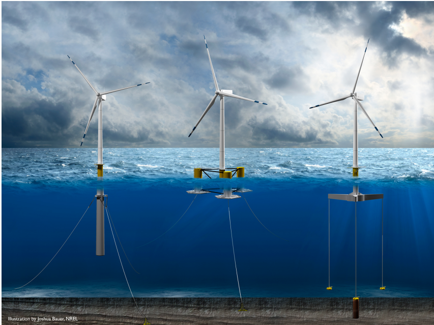
Figure 1.1: The three main floating wind turbine concepts: the spar (left), semi-submersible (center), and tension leg platform (right). Illustration by Josh Bauer, NREL.
