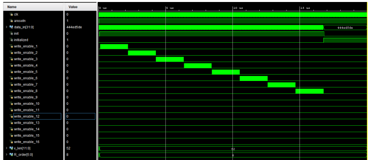
Figure 77: Waveform from simulating the Block ram module.
