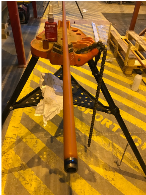
Figure E.16: Preparing drillpipe for connection
