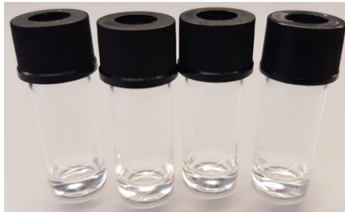
Figure 8: The sample glasses used for HPLC analysis loaded with 205 \mu\text{l} sample. After preparation the samples were stored at -20\text{ }^{\circ}\text{C} until they were analyzed.
