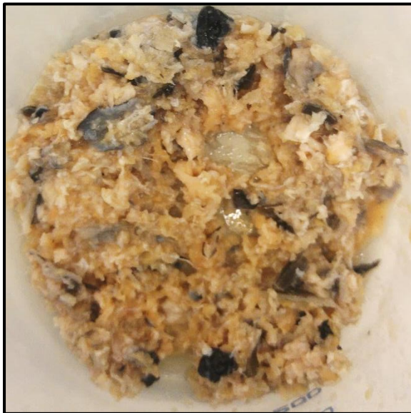
Figure 4: The raw material after all pre-treatment steps. In this form most of the low collagenous material is removed, like meat, fat and oil.
