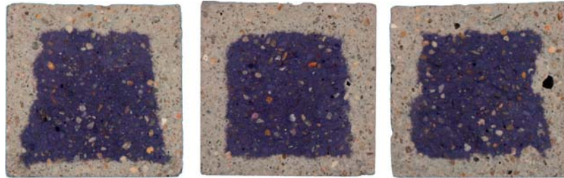
Fig. 5. Carbonation detection in the plain A' ( 40 \times 40 \times 160 mm) mortar samples. From left to right: cross sections of A'-J, A'-V and A'-T. The samples were sprayed with thymolphthalein after 8 weeks of exposure.
