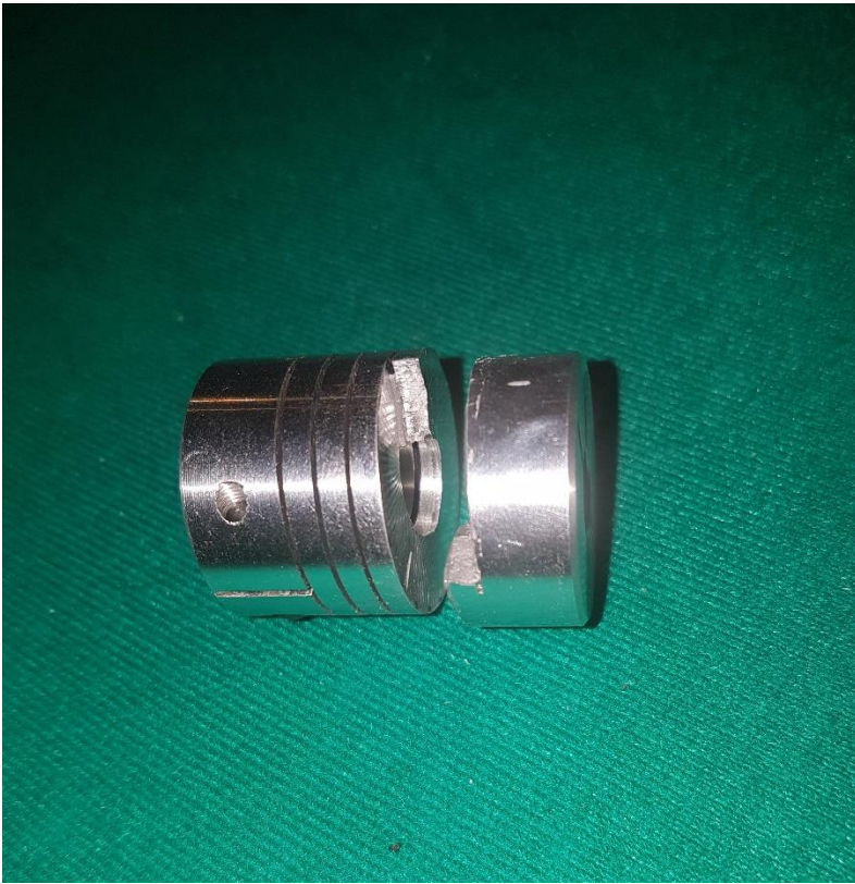
Figure 47. Broken motor coupling.
