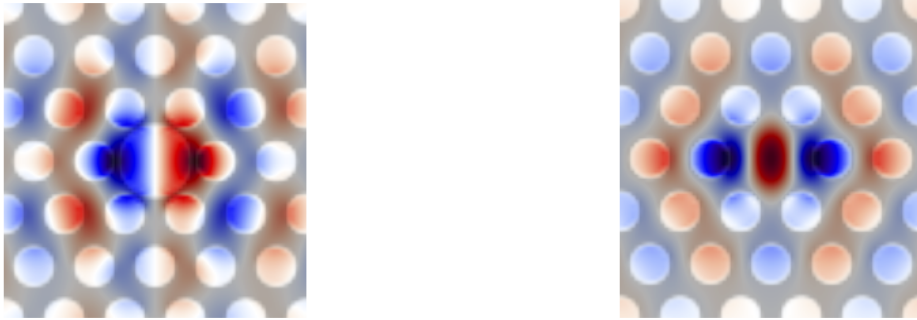
(a) Resonance mode "pulled" down from above the band gap, by increasing the size of the central cavity. (b) Resonance mode "pulled" up from below the band gap, by removing the central cavity.
