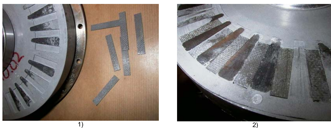
Figure 10.13 Test Machine 4. Insertion of slot wedges, 1) before slot wedge insertion, 2) after slot wedge insertion
