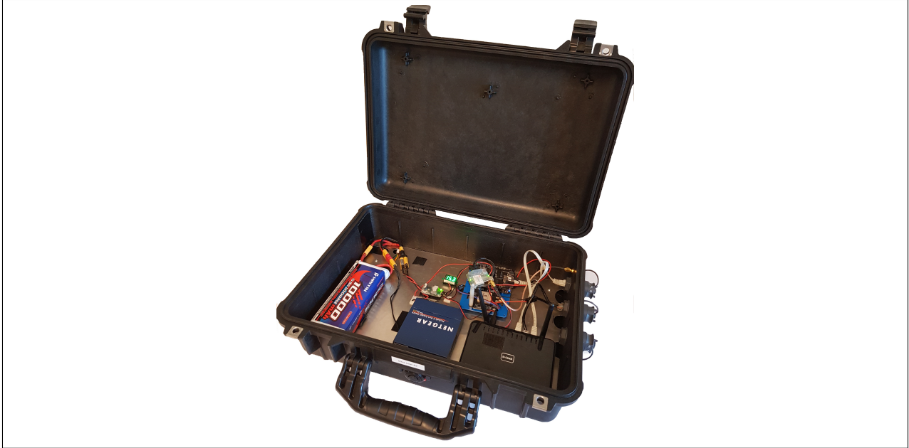
Figure 3.9: The base station components resemble the drone components, and provides the RTK GNSS correction data.
