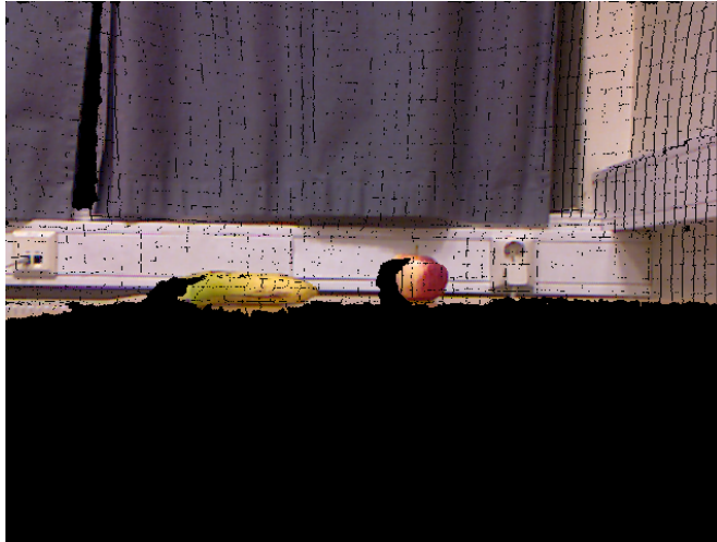
Figure 4.11: The RGB image taken by the Kinect was mapped onto to its depth sensor plane. For pixels in which the depth sensor had no information, the color is left black.
