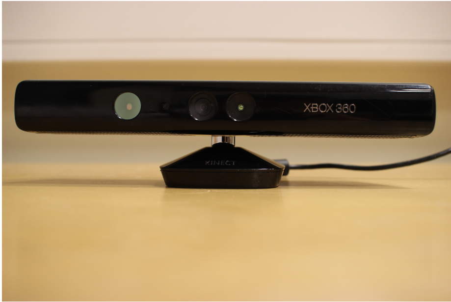
Figure 3.3: The Kinect. The three main sensors are visible behind circular glass covers. Left: IR light projector. Middle left: RGB camera. Middle right: IR light detector (depth camera).
