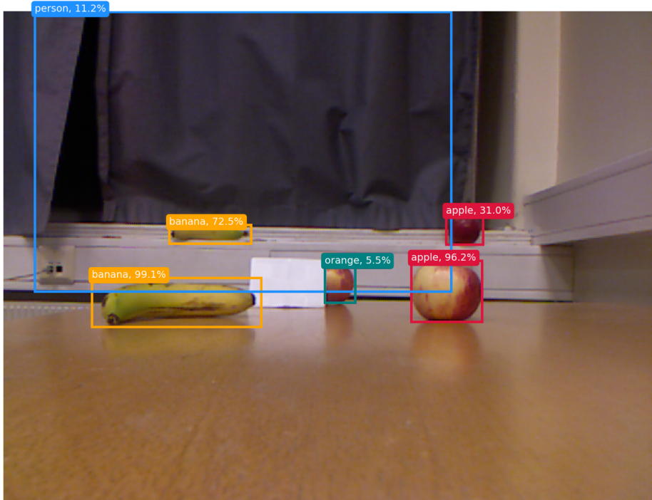
Figure 4.10: Apples and bananas were identified at different lengths away from the camera and being partially covered. The threshold was set to 5% in order to only reduce the most unlikely predictions. It is likely that the network mistakenly identified the curtains as a jacket or a pair of trousers, therefore labeling it a person. Another mistake was the prediction of an orange, that was in fact a partially covered apple.
