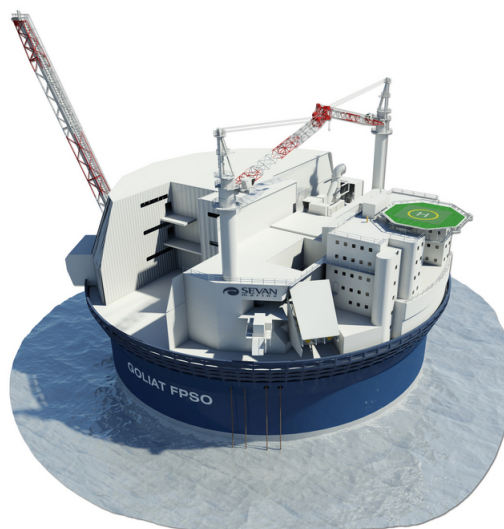
Figure 1.1: Concept drawing of the Sevan 1000 FPSO Goliat, from Steensen (2009)
