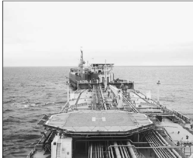
Figure 3.2: Tandem offloading seen from the shuttle tanker, from Chen & Moan (2004)
