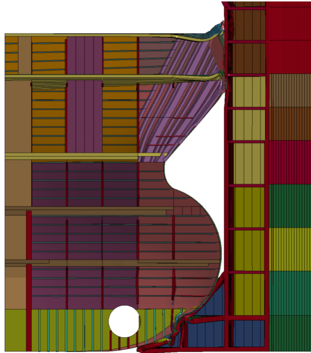
Figure 7.13: Crushing of FPSO bilge box and shuttle tanker forecastle in scenario 2
