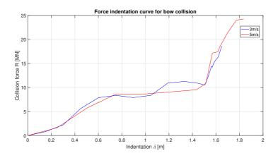
Figure 10.18: Comparison between force-deformation curves for forecastle in bow at 5m/s and 3m/s
