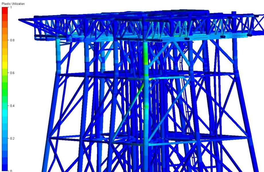
**Figure 11.14:** Plastic utilization after collision (Dynamic analysis)
