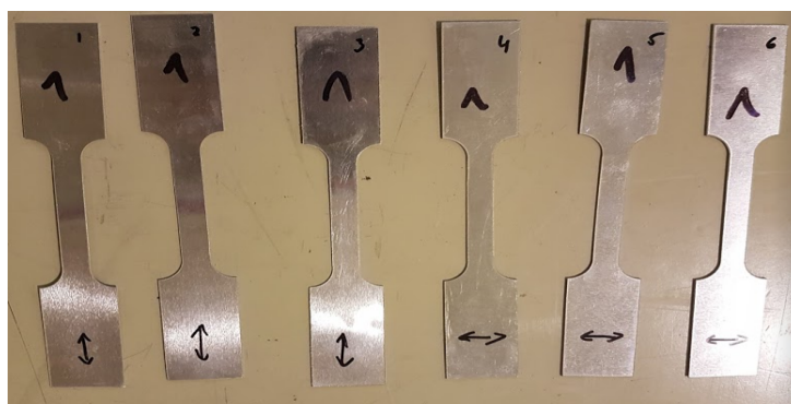
Figure 8.1: Tensile test samples nr. 1-6 of aluminium A1050 H111 with material 1 used in the tensile test
