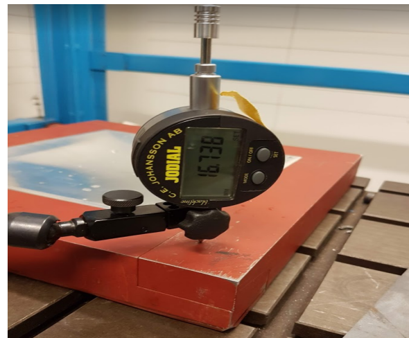
(b) Manual: Dial gauge measuring equipment
