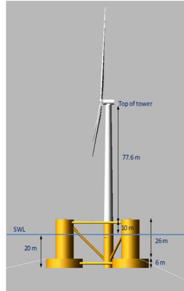
Figure 1 Side view of the OC4 DeepCWind semisubmersible wind turbine [5]
