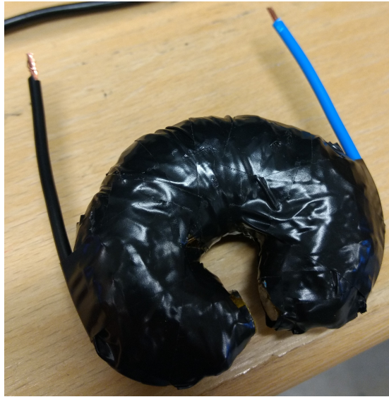
Figure 3.15: The home-made magnet with approximately 1200 windings, wrapped in heat resistant Kapton and electrical tape.
