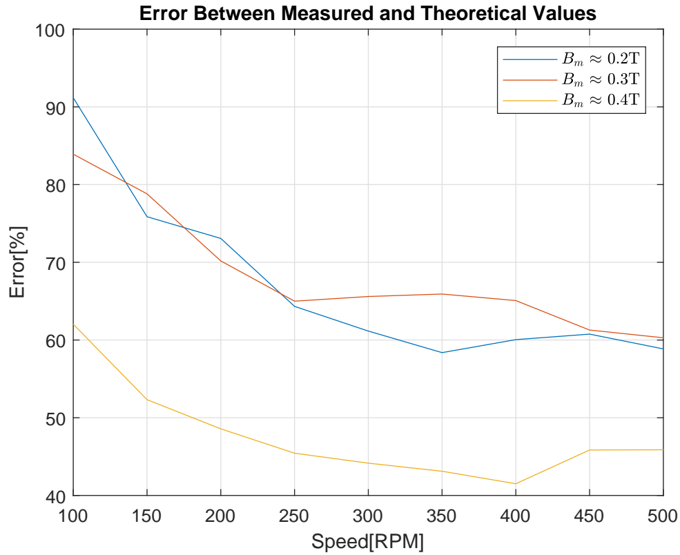
Figure 5.5: The data collected from the permanent magnet also show the error to converge as the speed, and thus torque, increases.
