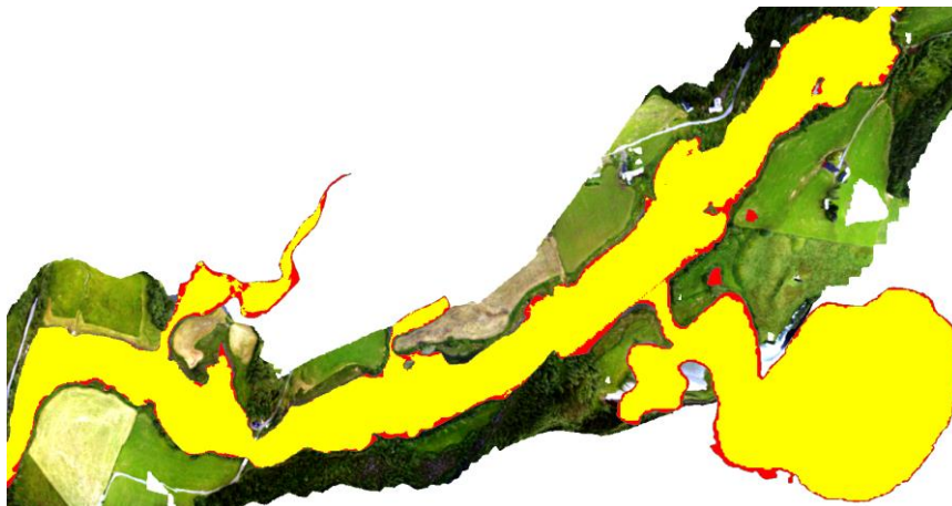
Figure 5-11. The comparison of the observed and computed water-covered area
