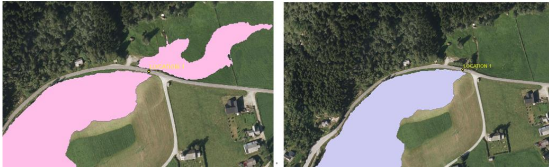
Figure 5-20. The flood extent with different mesh resolution.
